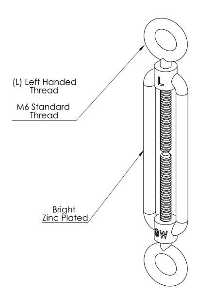
MODEL No. / 419 Forged Straining Screw Eye to Eye 6mm
