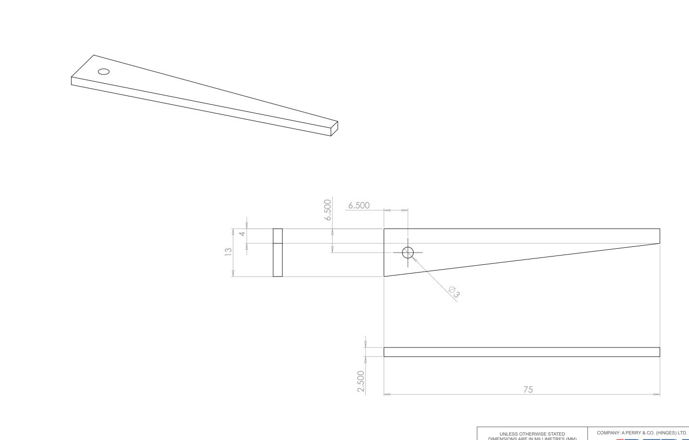
UNLESS OTHERWISE STATED DIMENSIONS ARE IN MILLIMETRES (MM)
